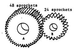
Answer: ... The gear at right will turn twice as fast as the gear at the left and in the opposite direction. So we could say that the right gear turns -2 times as fast as the left gear.
